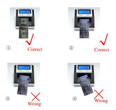
After a note was inserted, the detecting system will check it and then alert the user with an audible signal, indicating whether the banknote is genuine one or fake one.
