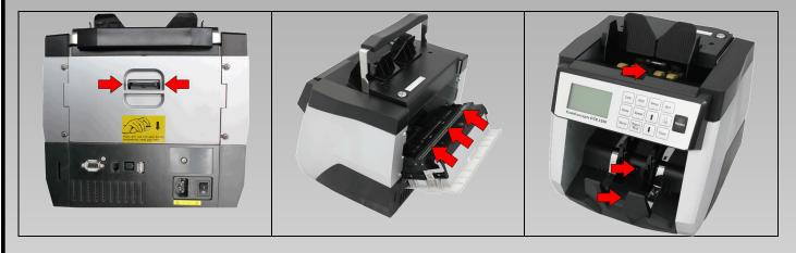
To open the CCE 3200 press on the back the button of the rear flap to get access to the sensor bars. Use a soft brush and cloth to remove the dust from the sensors, as well as from the feed rollers. To clean the counterfeit sensors we recommend the additional use of a non-flammable compressed air spray, so even in inaccessible places dirt and dust can be removed.
